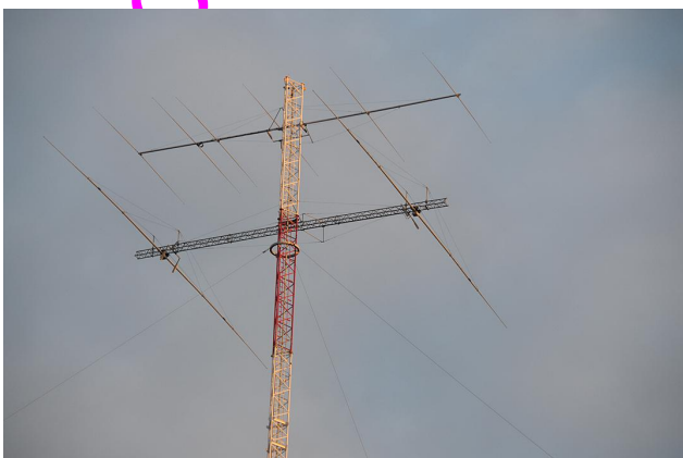
What is called “the upper 80-m 2-el yagi”. In WPX CW the sun is only 4
