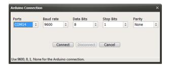
11. Clicking on the Connect button will allow access to the main form for QSO entry and access to menus.
